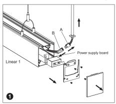
Install the Linear 1 to the ceiling as instruction of Suspension Installation. Open the end cap as the picture shows.
