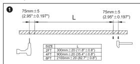
Drill a hole of 5.0mm in diameter as shown in the figure at the location required forinstallation. Then hammer the plastic anchor
